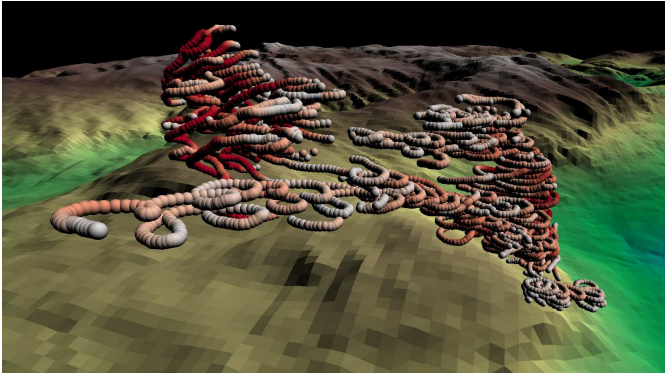
Fig. 4: A 3D view of an examined thermal. The thermal has been segmented and clustered from flights of multiple pilots in the same location spanning a short time-interval of about 15 minutes. The thermal is colour-coded by the vertical velocity. The topographic map is colour-coded by altitude. In this particular case we see two clusters that were incorrectly clustered into a single thermal. The domain experts need to take this into account when modelling.
