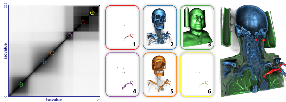
Figure 3.6 – Representative isovalue selection algorithm applied to a CT data set. The isosurface similarity map is shown on the left and the six most representative isovalues are marked. The corresponding isosurfaces are depicted in the middle section numbered from one to six with decreasing relevance. The image on the right shows a cutaway view of the data set classified according to maximum similarity with the six isovalues.
