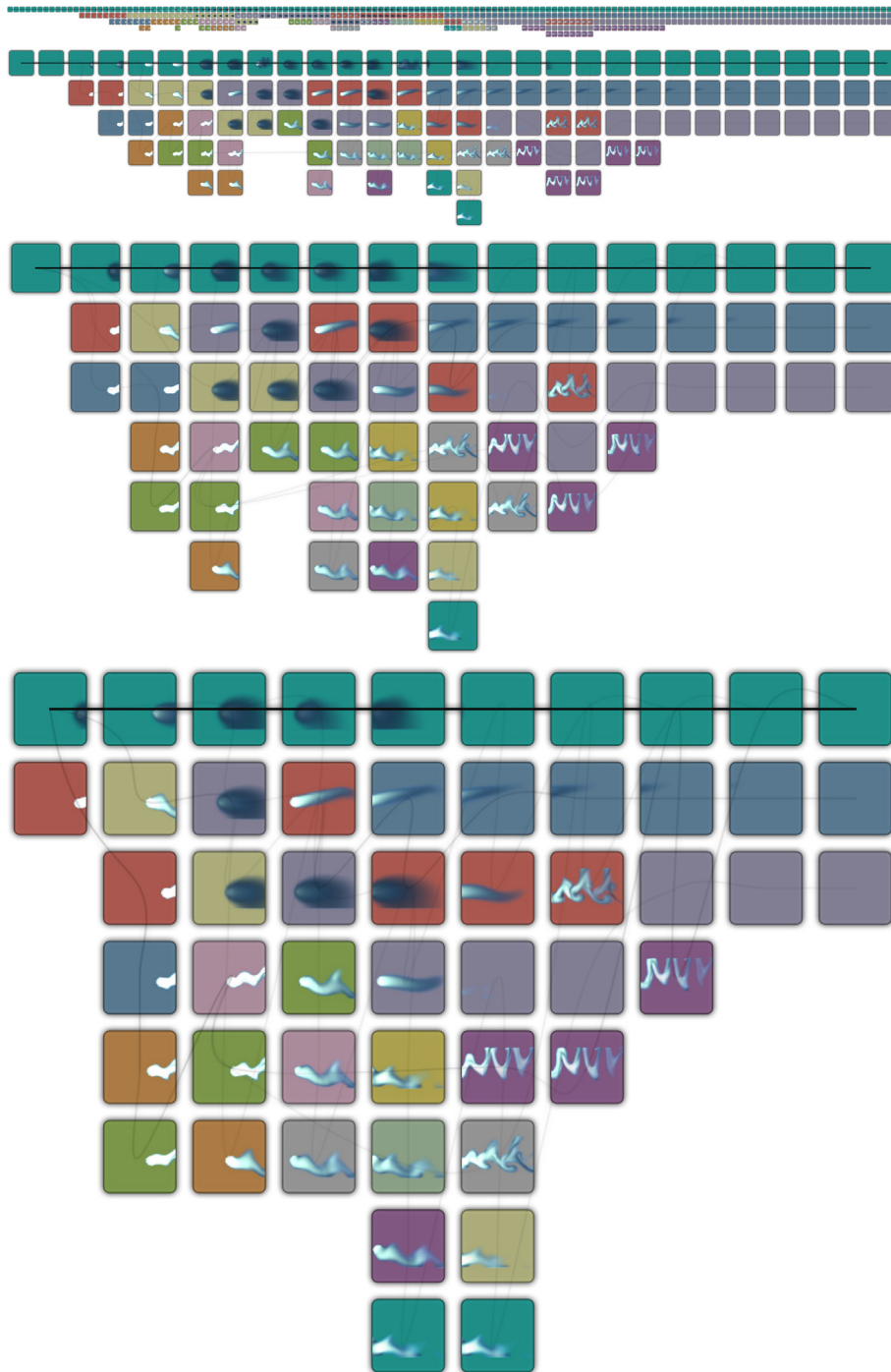
Figure 6.4 – Cluster timeline at different temporal compression levels. The depicted time interval sizes are, from top to bottom: 1, 5, 10, and 15. The sequences in this set of 128 simulations of a bullet passing through a medium have 150 time steps each.
