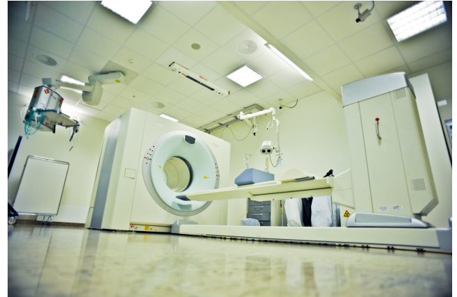
Figure 3: A PET/CT scanner developed by Siemens Healthcare. Photo courtesy of the Centre for Nuclear Medicine and PET, Dept. of Radiology, Haukeland University Hospital in Bergen, Norway.
