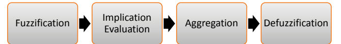
Figure 5: Workflow of our FIS. First, crisp input values are fuzzified using fuzzy membership functions. Second, the antecedents of the if-then rules are evaluated using fuzzy set operators. The implications are evaluated with the minimum operator [15]. Third, the fuzzy implication results are aggregated and, fourth and finally, defuzzified using the centroid method to provide a crisp output.
