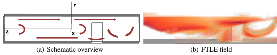
Fig. 5 (a) Schematic overview over the flow domain, z being the streamwise direction. (b) The FTLE field of a simulation of a bursting dam with parameters t_0 = 62 and T = 68 . The FTLE values greater than 0.25 are brushed (smooth lower bound 0.2). We see that we can identify expected structures around the obstacle. The upper rear part of the flow domain shows large regions with high FTLE values, presumably induced by shearing.
