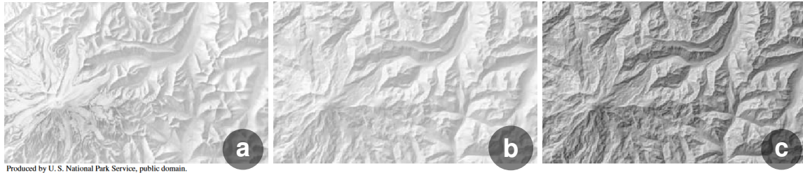
Figure 2.23: Comparison of (a) a hand-drawn shaded terrain relief and (b,c) two results of exaggerated shading for depicting shape and detail by Rusinkiewicz et al. [139].
