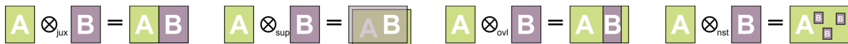
Figure 2.1: Overview of four composition strategies according to Javed and Elmqvist [87]. From left to right: juxtaposition, superimposition, overloading, and nesting.
