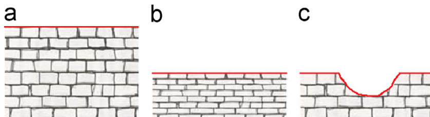
Figure 3.3: (a) Texture on the initial configuration of a layer; (b) compacted layer which is communicated by a compacted texture; (c) eroded layer which is communicated by a cut texture, where no texture deformation is performed. Image courtesy of Endre Lidal [73].
